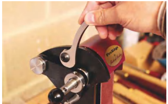
▲ A substantial cam lever applies the belt tension
